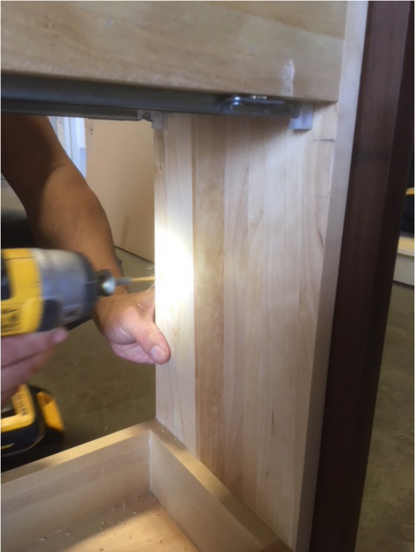
Drill holes on drawer face before use screws to prevent cracking.
