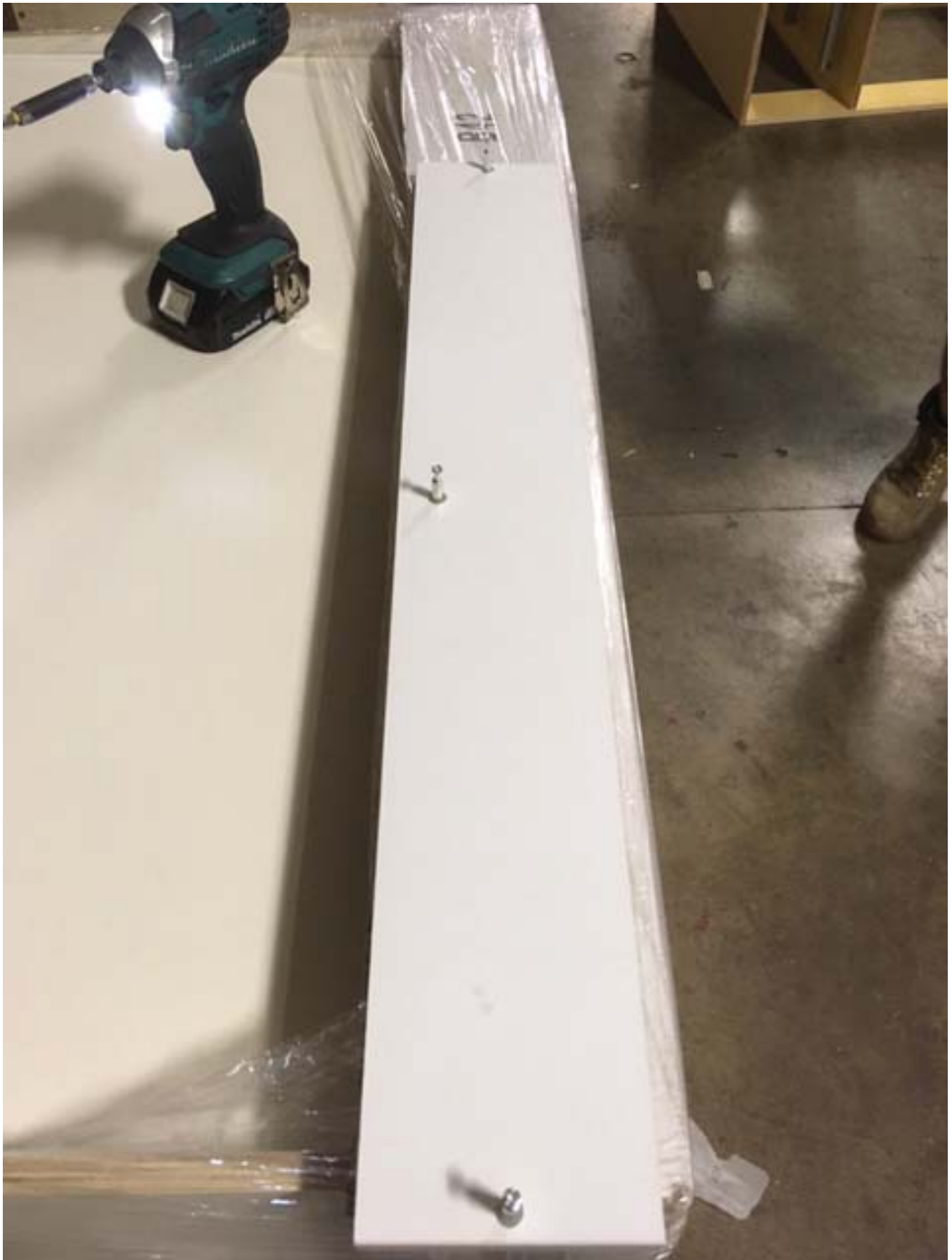
Attach cam-lock screws to pre-drilled holes on the kick board.
