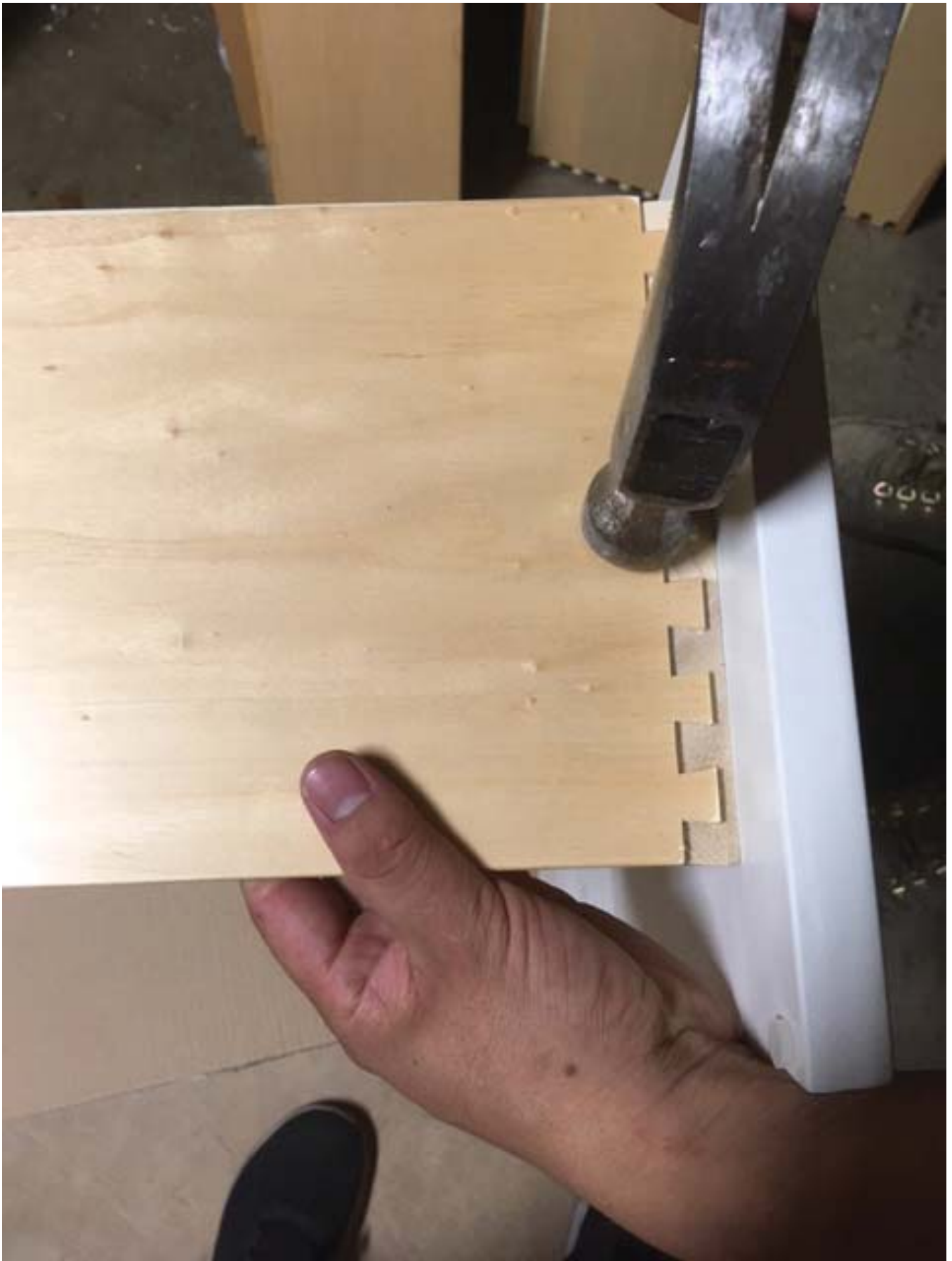
Hammered the dove-tailed drawers; use nail gun to give extra strength.
